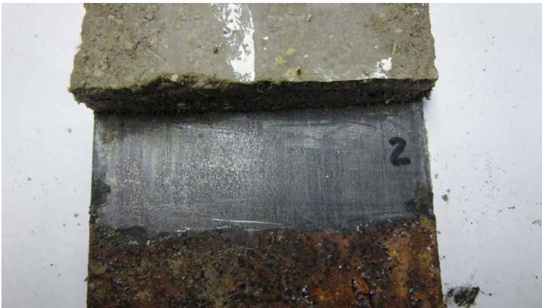
Insulated metal panels after 2000 hours of exposure
