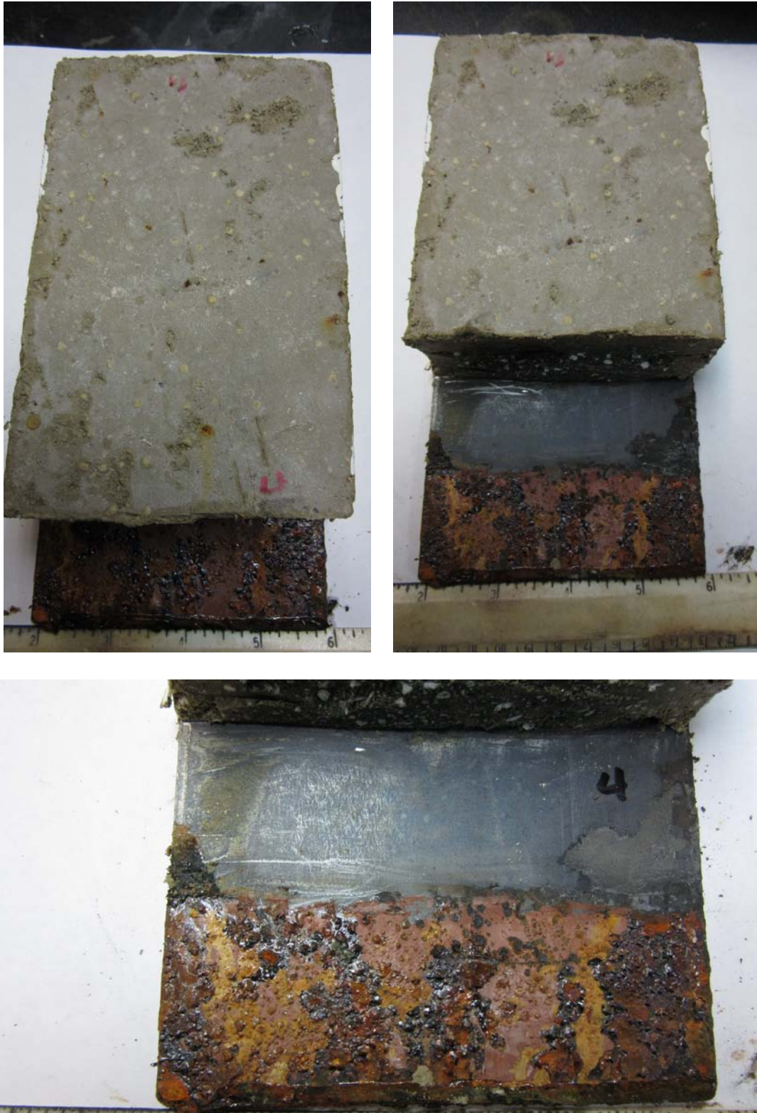
Insulated metal panels after 2000 hours of exposure
