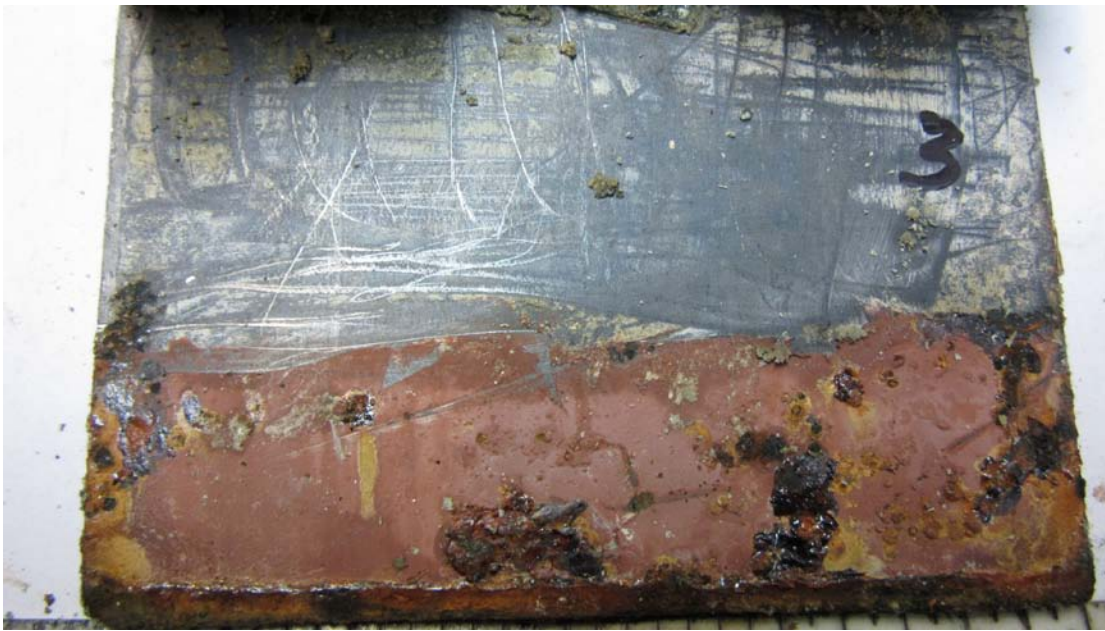
Insulated metal panels after 2000 hours of exposure
