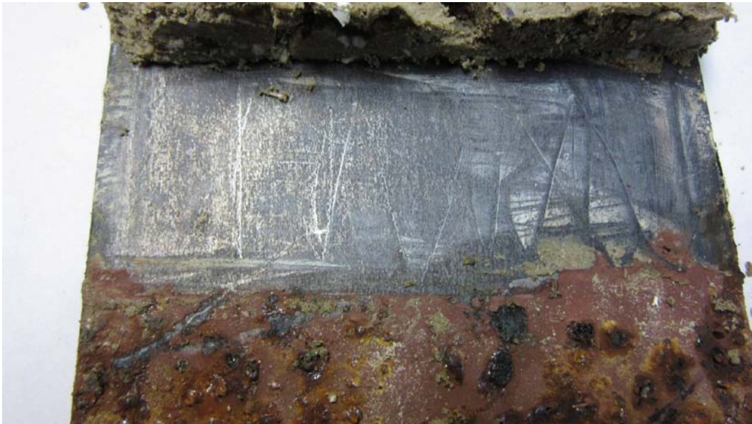
Insulated metal panels after 2000 hours of exposure
